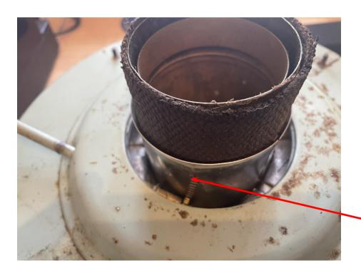
Carrier moves about 5mm up and down but wick is stuck to tube.
